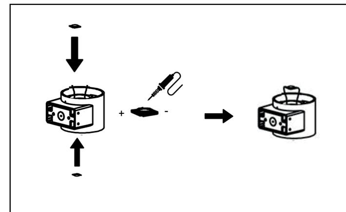
4. To connect the new chip with driver output cable by soldering machine. The red cable from the driver should be soldered to the + pole of the chip, and the black cable should be soldered to the - pole of the chip.
