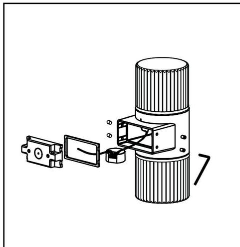
2. Loose the screw by wrench, to take the bracket and driver out.
