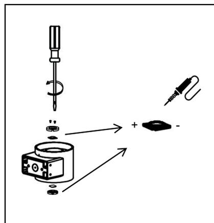
3. Remove the lightsource bracket by screwdriver and melt the + - poles of LED chip by a heated soldering machine to take out LED chip.
