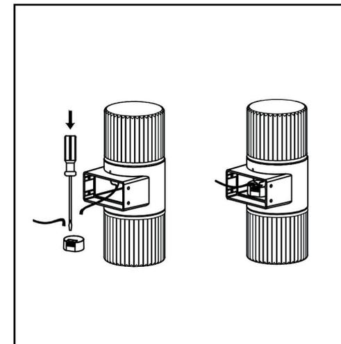
4. Press the driver button by screwdriver and put the new driver cables in it to complete the connection.
