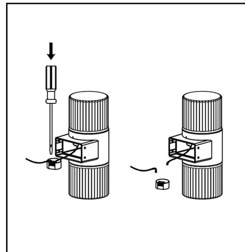
3. Press the driver button by screwdriver and take the driver cables out.
