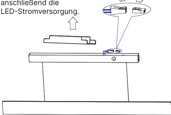
④ Connect male and female plugs, and install the LED power supply in the lamp housing.
