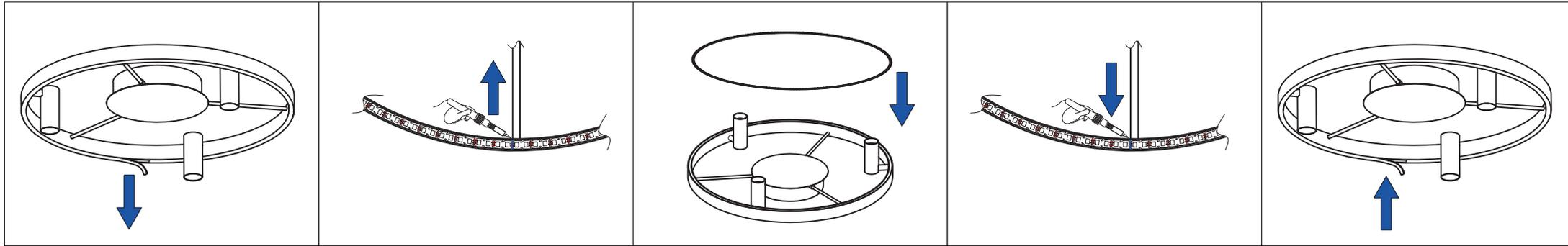
1.Remove the silicon diffuser.
