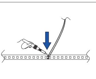
5.Connect the wires and LED strips with a soldering gun.
