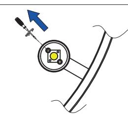
9.Remove the screws with a screwdriver. Remove the light source.
