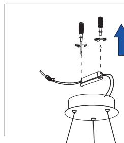
13.Remove the screws with a screwdriver.
