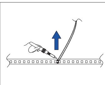
2.Remove the wires from the LED strip by soldering gun.
