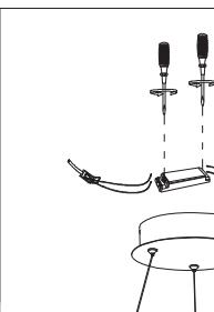
14.Remove the wires from Driver.
