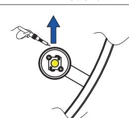
8.Remove the wires from the light source by soldering gun.
