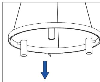
1.Remove the silicon diffuser.
