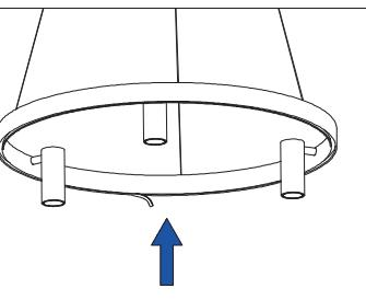
6.Install the silicon diffuser.
