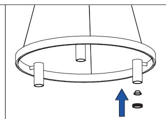
12.Install the lens, rotate and twist on the cover.
