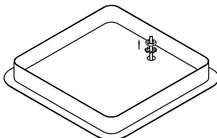
⑥ Remove the fixing nut of the spotlight from the base and remove the lamp head
