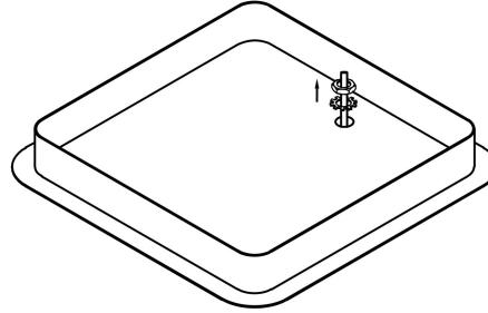
②Use nuts to regulate the lamp head onto the base
