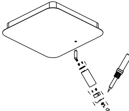
⑦ Remove the COB light source fixing components inside the spotlight, welding off the old COB
