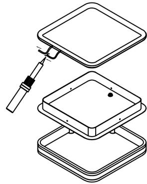
⑤Stick the LED strip on the base and welding up with the cable,reinstall the silicone strip
