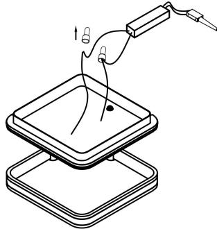
⑦Reconnect the driver and wires with nipple connecting
