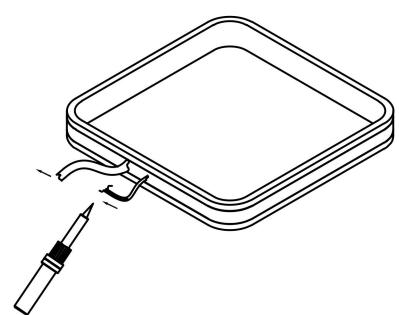
③Stick the LED strip on the aluminum frame and welding up with the cable,reinstall the silicone strip
