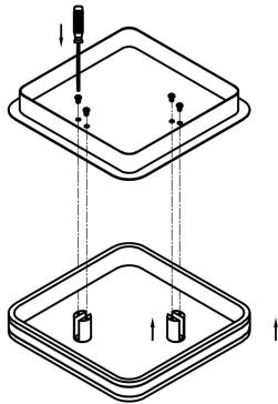
④screw up the fixing components connecting the base and aluminum frame
