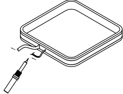
③ Remove the silicone strip from the aluminum frame and welding off the old LED
