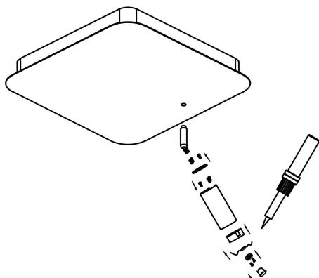
①Install COB light source fixing components inside the spotlight an welding up the new COB with cable
